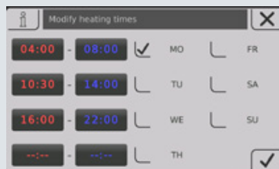
Fig. 2 View of the heating times (individually adjustable)
